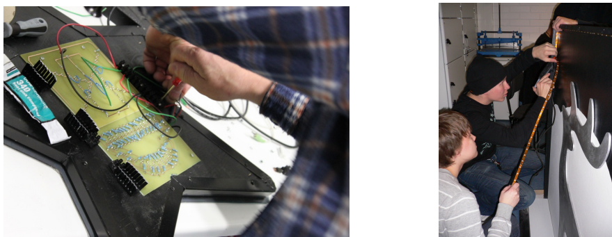
Figure 3. Circuit board and RGB- led- ribbon installation
